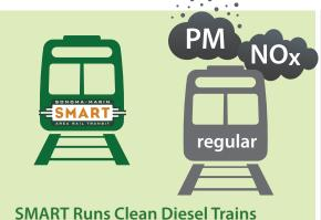
SMART's clean-diesel trains have modern, efficient engines that meet the EPA's Tier 4 emission standards, cutting particulate matter emissions by 96% and NOx emissions by 93% compared to regular diesel engines.
